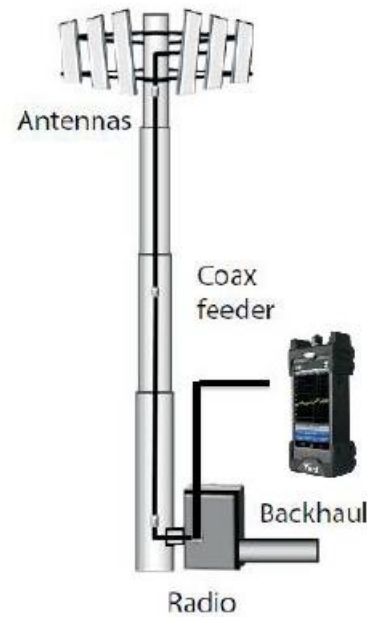
Conventional cell site
